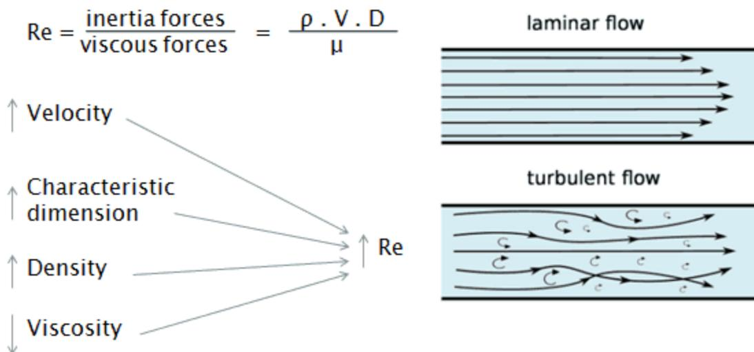
Figure 1 Laminar vs. Turbulent Flow
