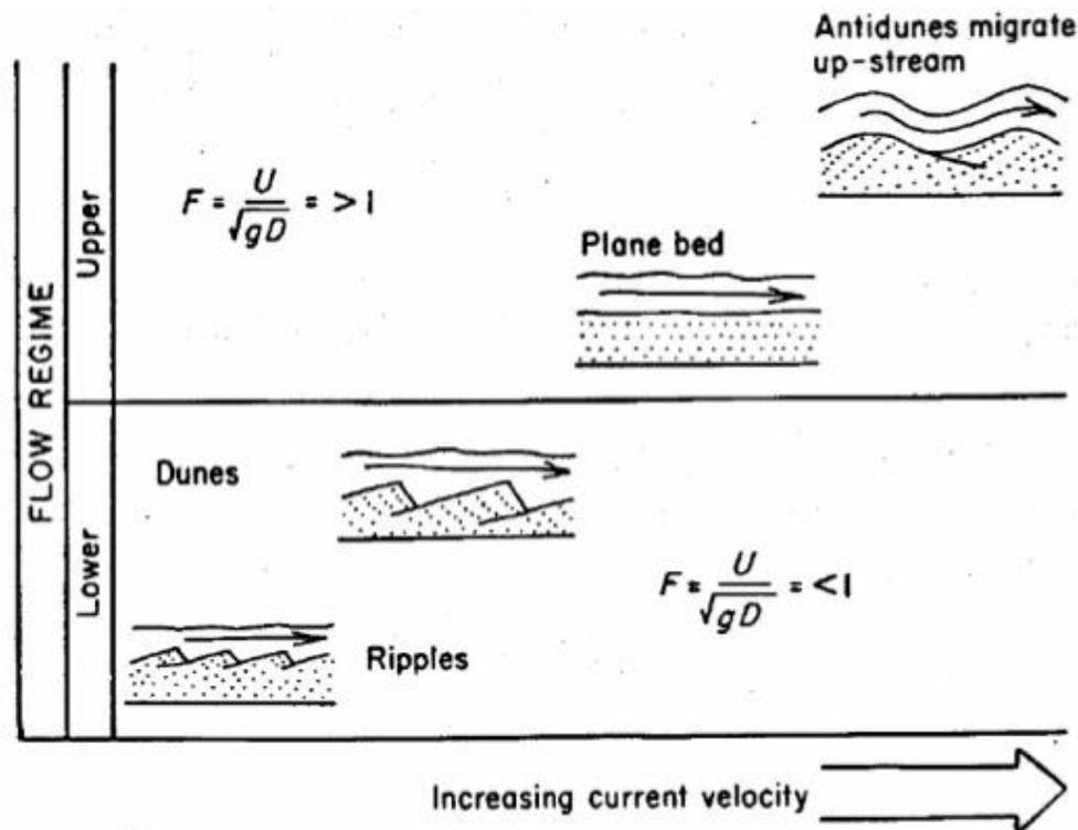
Figure 2 Bed forms and sedimentary structures for different flow regimes
